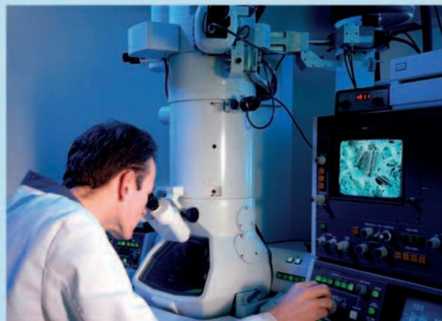
▲ **ELECTRON MICROSCOPE** *A scientist looks at a 3-D image created by a scanning electron microscope. The same image can be viewed on the monitor's screen.*
