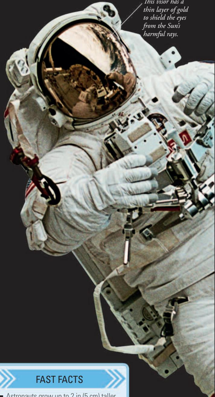
*This visor has a thin layer of gold to shield the eyes from the Sun's harmful rays.*
